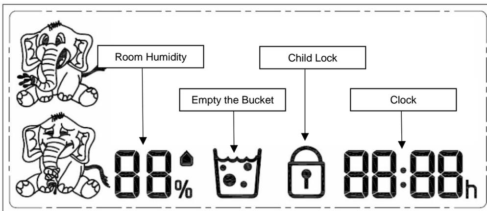
The above is all you need to do for day to day operation. The current relative humidity and temperature within the room is displayed at the bottom left of the display.
