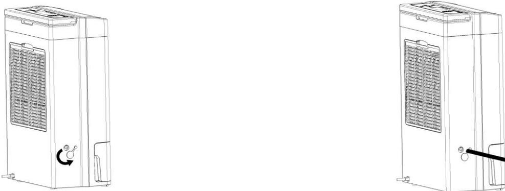
2. Remove the bucket, push back the drip stopper and push the hose onto the water outlet.
