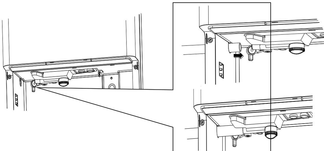
3. Reinsert the bucket and make sure that the hose runs downhill.
